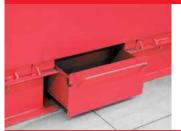
The machine frame is designed to easily collect the dust generated during the straightening process and also it is sound proofed to achieve maximum noise reduction during operation.
