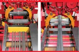
• The automatic tying unit aligns and ties the cut to length bars.
