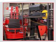
Pre-straightening and feeding unit equipped with winch and pre-straightener with motorized roller, available on METRONIC 20 model, eases and speeds up the alignment and the insertion of the wires.
