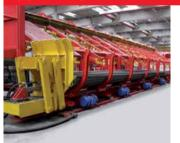
The guiding support is available in several versions, allowing the collection and distribution of straightened bars according to specific production needs. The version that includes the automatic alignment device (optional) is particularly suitable for the production of bundles intended for welded mesh equipment.
