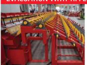
• Evacuation bar system with tipper and mobile star rack is a unit that collects, transports and deposits the cut to size bars by creating an efficient intermediate storage station. (OPTIONAL)
