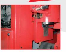
A hydraulic shearing unit of extremely robust design, which is capable of performing a complete cutting cycle in only ~0.1 s (Metronic 10–13 HS Plus). This solution allows processing at high speed within the required measurement tolerances. The unit is also equipped with cutting blades which can be used on all of their edges, for a total of 8 different cutting surfaces.
