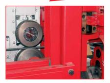
The extraction pulling unit (Metronic 16-20) reduces the scrap and eliminates the downtime needed for the extraction of the "tails". The final section of the coil is straightened and extracted fully automatically.
