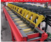
The "support and alignment chains" can be equipped on request (optional) with a device for lifting the bars, integrated with one motorized roller conveyor
