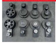
• MULTIRADIUS 36 BEND is equipped with a series of self-locking bending pins (patented) with self-locking fastening. The pins are made in compliance with international regulations and are quickly replaced when changing the diameter, allowing an immediate restart of production.
