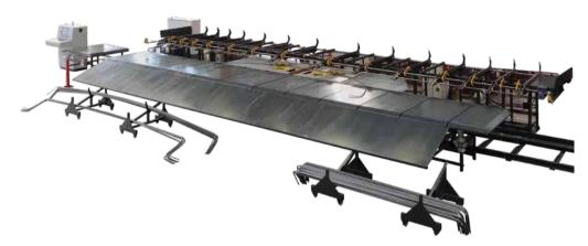
• The two bending and calendering heads are positioned parallel and near to the mobile collection stations. In this way it is possible to divide the products according to their processing position (tag) using the entire length of the worktop.
