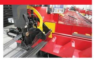
device aligns the bars before they are counted and loaded into the machine, guaranteeing correct measurement tolerances. A magnet draws and counts every single bar with extreme precision, avoiding counting errors (loading one bar instead of two) which would distort the quantities to be produced, as well as compromising the optimization already programmed.
