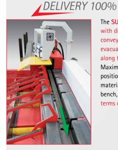
The SUPERFLEX is available in versions with different numbers of distribution conveyors that can be loaded from the evacuation channel in any position along the full length (12, 14,...m). Maximizing the number of available positions for intermediate collection of material before delivering out of the bench, provides an enormous benefit in terms of optimization of cutting list.
