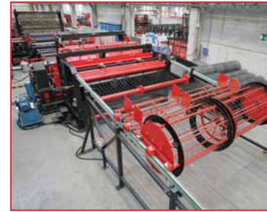
Buffer station of mesh in coil.
