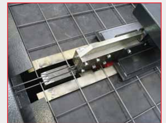
Longitudinal cutting unit for mesh produced to form two rolls.
