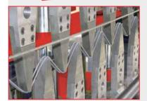
The continuous chain forming device (zig-zag) comprises a pair of chains which bend the two diagonal wires. The exclusive system allows independent control of the forming of the two wires during the feeding and shaping process, so that any difference in section or mechanical characteristics between the two wires can be taken in account. In this way the lattice girder will always be well formed with excellent symmetry and straightness.
