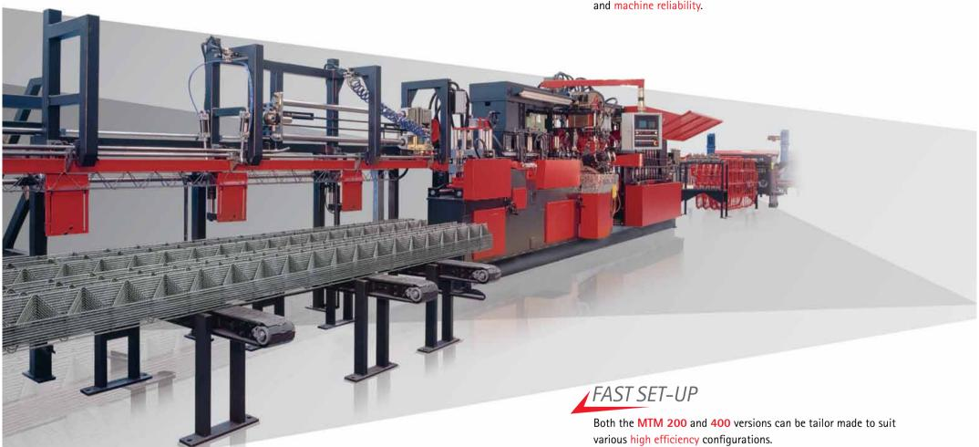
These are suitable for a variety of production scenarios whether producing large series of standard lattice girders or manufacturing a mix of different sizes and dimensions.
