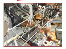
The use of latest welding technology (controlled current profiles) overcomes variations in the mechanical characteristics of the steel material, whilst assuring reduced power consumption.
