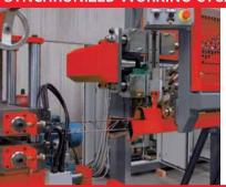
• The automatic transfer device of the lattice girder comes into operation after the cutting operation, thus enabling the production of next section.
