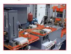
The feeding group is perfectly synchronised with the chain forming group so that the lattice girder will be produced in perfect symmetry.
