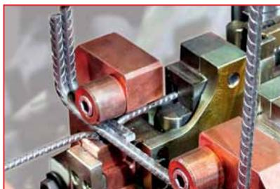
The cutting units (patented system) allow cut to length the longitudinal wires, **eliminating manual operations and the relative waste.**
