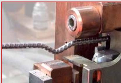
The "V" shape of the **longitudinal wires** (patented system) allow to keep them **inside the stirrup structure**. The obtained **pre-cage** therefore **complies with the designed standards** and is much more **rigid**, then the following handling will not deform the structure.
