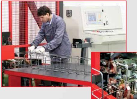
The **lateral positioning** of the stirrups on the welding heads allows a **simple, fast** and **safe** loading. The three welding heads allow the maximum freedom in positioning the electrodes, between stirrups and longitudinal wires. It is possible to use **stirrups of different diameter wire**, arranged automatically with **fix or variable pitch**.
