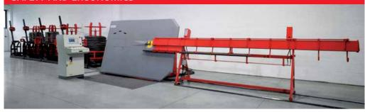
With the system it is always granted to obtain closed stirrups, thus eliminating the typical and dangerous manual operation during the bending process by operator.
