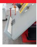
"TFS" allows to obtain always closed stirrup, eliminating the dangerous manual intervention of the operator during the bending phase. The exclusive design of the worktop, equipped with a lower collapsible element, makes it possible to produce large stirrups (maximum distance between the central pin and the flooris 1900mm) as well as becoming a collection shelf for all the stirrups, thus avoiding their fall to the floor.
